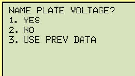
Press the **[3]** key if you would like to use the name plate voltage values from the previous test performed. **Continue to step c.**
