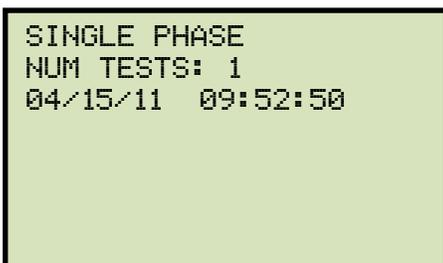
Press the [**Contrast** √] key. The test record details will be displayed as shown below:
