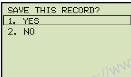
Press the **[1]** key (*YES*) to save the test record to the unit's Flash EEPROM.
