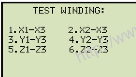
Select the winding by pressing the corresponding numeric key on the keypad.
