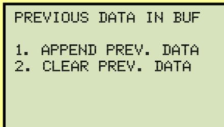
Press the **[1]** key (APPEND PREV. DATA) to append the data in the unit's working memory to the current test results, or press the **[2]** key (CLEAR PREV. DATA) to clear any previous data from the unit's memory buffer and only save the current test results.
