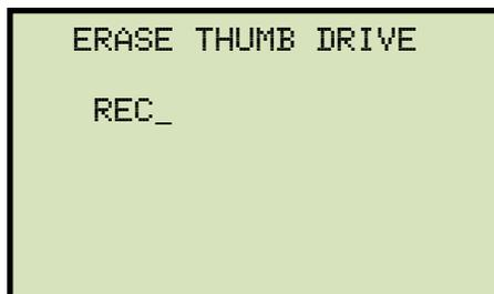
Type the record number that you would like to erase using the alpha-numeric keypad and then press the **[ENTER]** key. The test record will be erased from the USB Flash drive and the following screen will be displayed:
