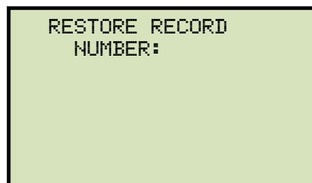
Type the record number using the alpha-numeric keypad and then press the **[ENTER]** key.
