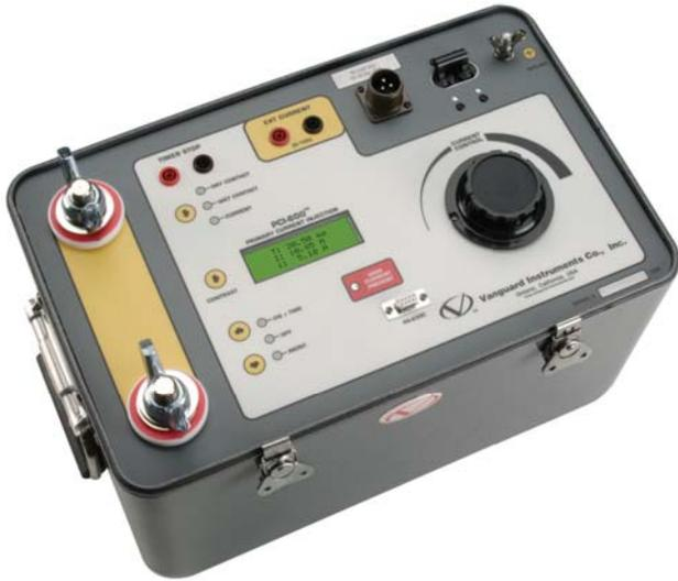
The PCI-600 is a programmable AC high-current source designed specifically for utility-substation applications. This device is well suited for primary injection testing of protective relays. This versatile device can also be used for testing thermal, magnetic, and solid-state motor-protection relays and molded-case circuit-breakers, as well as any application that requires a high-current source.
