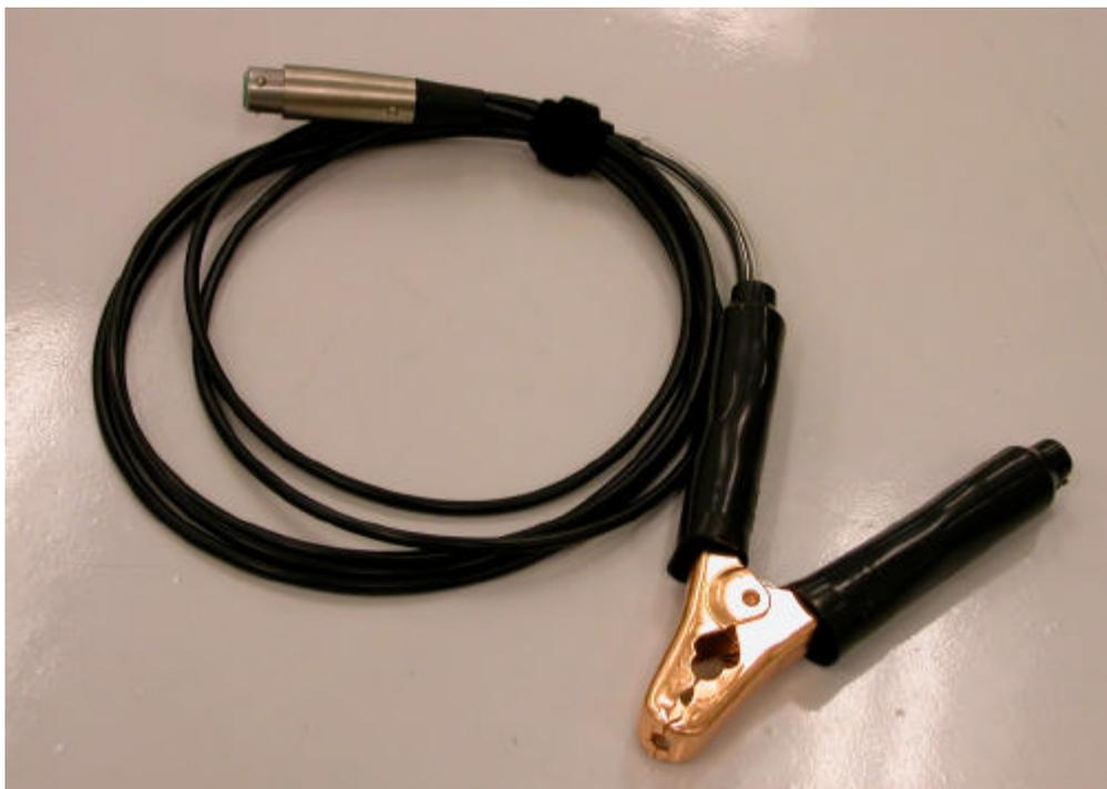
**Figure 2. High Voltage return cable**
